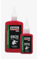
It is a high-strength retaining compound that developed especially for passive surfaces. It has a resistance to hot oil. The product is applied between metal connections and cures by reacting in the absence of air. It works well on cylindrical parts to be assembled even if there is a slightly dirty surface.
