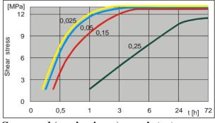
Cure speed (on aluminum) vs. substrate
